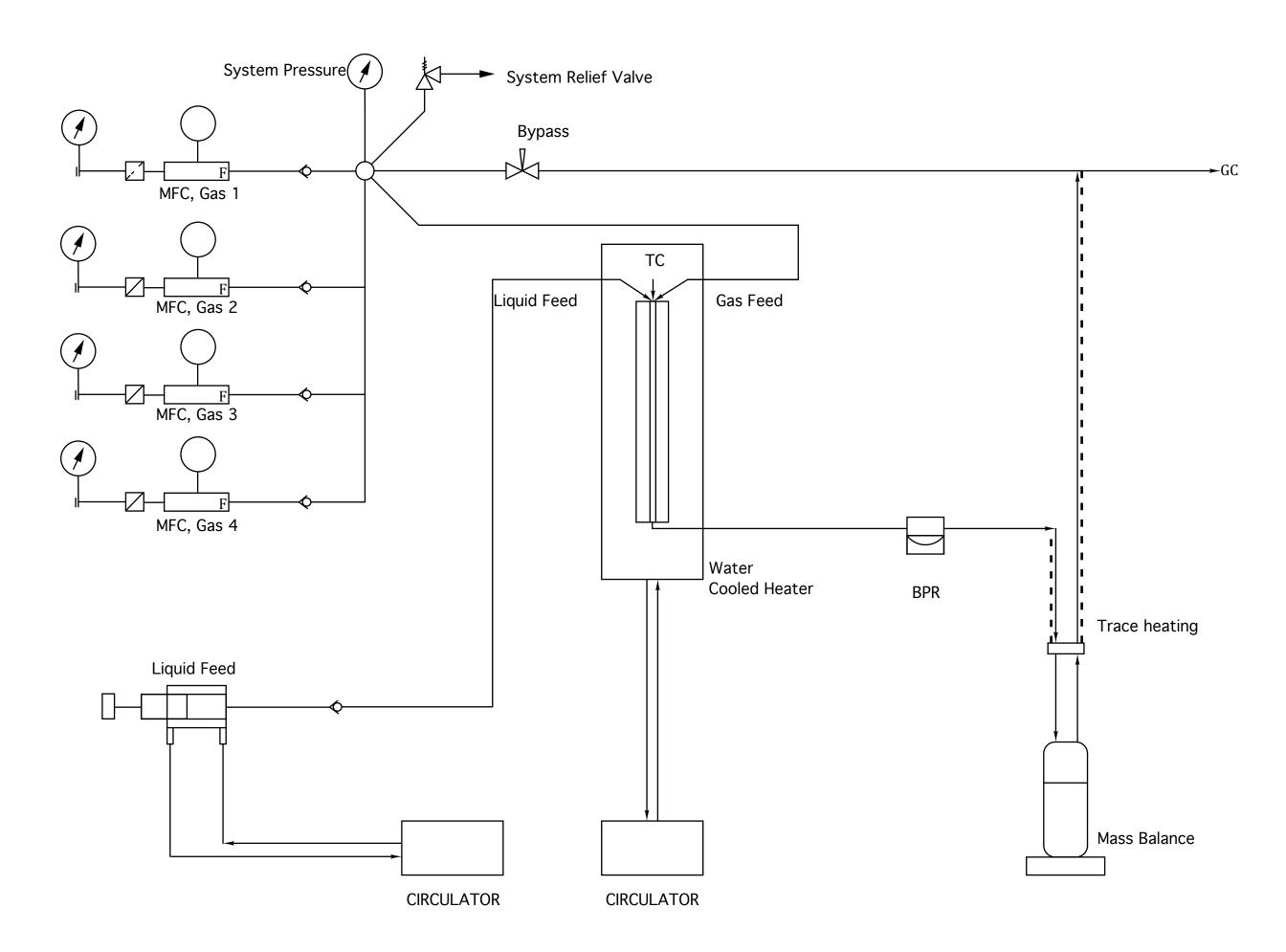
CAMBRIDGE REACTOR DESIGN LTD SCHEMATIC. FIXED BED REACTOR - ADVANCED SPECIFICATIONS. 100 BAR, 500C.
